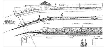
To improve safety for both vehicular and pedestrian traffic, GEC consolidated and removed driveways and altered parking encroachments along the corridor for improved access management principles.
